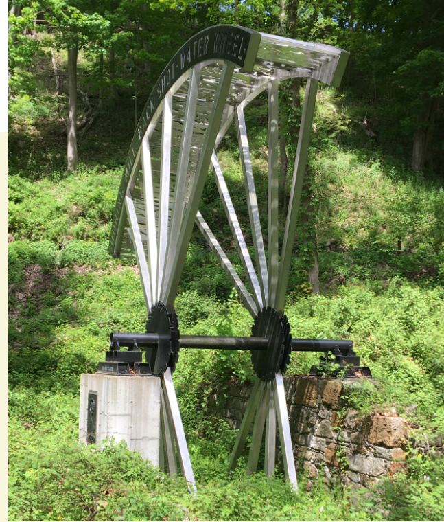
Fig. 11. C&G Partners used marine-grade stainless steel to create a durable replica of an industrial water wheel at the West Point Foundry Reserve in Cold Spring, New York.
