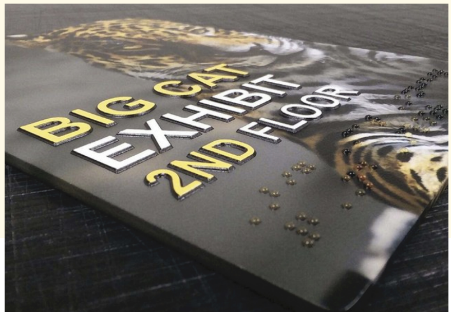
Fig. 5. Powder-coated graphics were used for this tactile sign with dimensional text and Braille letters, created as a test sample.
